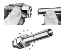
Hold the fitting body steady with a backup wrench and tighten this nut 1¼ turns. Watch the scribe mark, making one complete revolution and continue to the 9 o'clock position.
